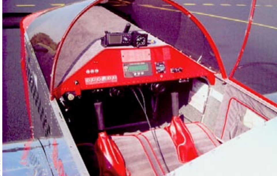
Spicer's Grand Rapids EIS displays airspeed and other flight information. The rectangular placard above the EIS is his checklist.
